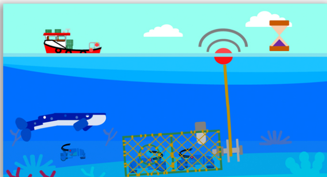
5. Buoy will release at time. Location transmitting to Onboard Gateway
