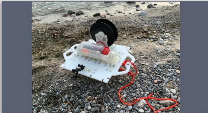
3. Install Buoy to Release Mechanism and attach to gear
